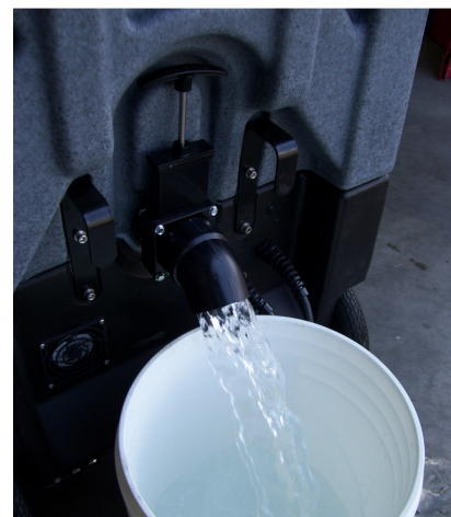
Drain water from Recovery Tank
