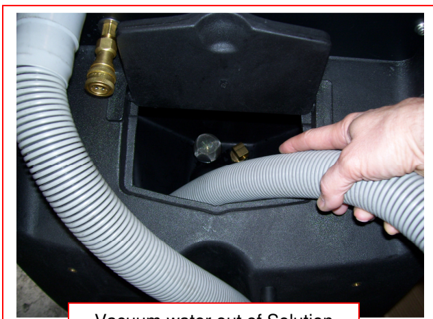
Vacuum water out of Solution Tank
