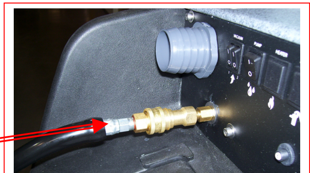
Connect the male end of the HP Solution Hose Assembly to the female solution outlet fitting on the machine. Connect the female end to the cleaning tool.
