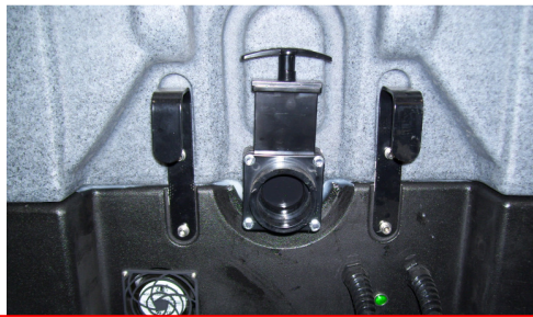
Remove four bolts holding valve assembly to flange fitting
